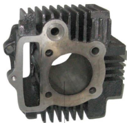
inner cylinder wall
